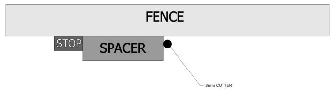
Now cut a piece of scrap MDF to the exact length as your box and make a test cut. If everything is carried out correctly the lock should be a great fit. From this test cut you can also check the router bit depth of cut fitting your lock plate in and ensure that it is perfectly flush - and that the fence is the correct distance from the bit. Now cut the mortises for top and bottom.
