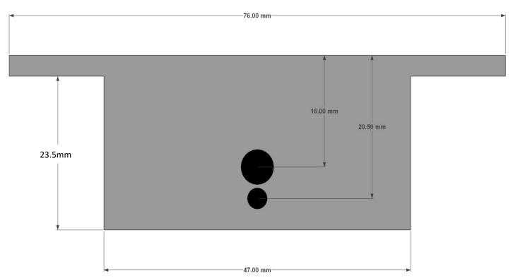
Remove your lock and add a piece of scrap to the case mortise with the same thickness as the lock case. This will prevent tear out when drilling the following holes. Drill your 3mm hole first and then the 5mm hole and joint up using a jewellers file. Complete the process by shaping the keyhole for a more traditional look or leave as is.
