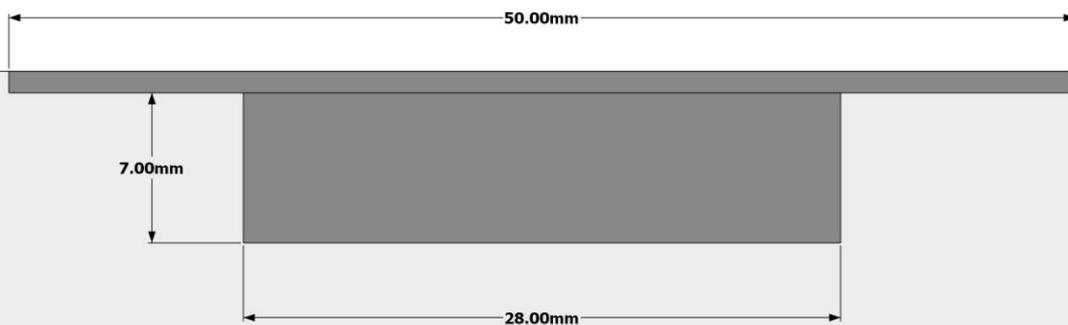
The lower part of the catch needs some chisel work to allow for the action to work - please see above. The upper part of the catch has a piece on the reverse that sticks out. You will need to chisel out a piece on the lid of your box to allow this to sit in flush. Once done square up the corners with a sharp chisel. Next drill your holes, fit the screws and you're done!
