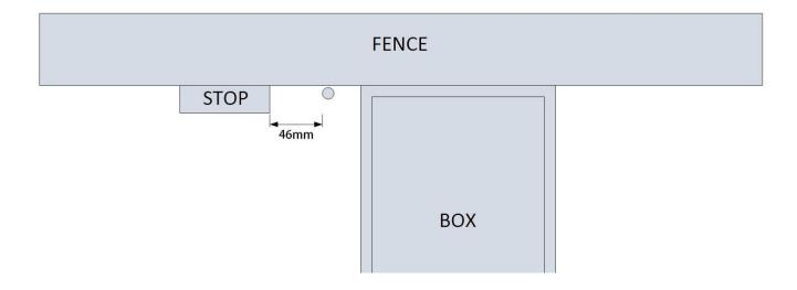
If you do not want a gap, then the depth should be exactly half the barrel thickness. Once these are cut, set an opposing stop up the same way for the other 2 mortises.
